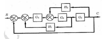
2. Simplify the following diagram using block diagram reduction method. Also derive the transfer function of the same using signal flow graph.(15) (A)
