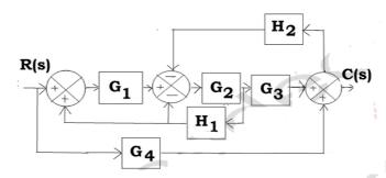
9. Illustrate Masons formula to derive the transfer function of a given SFG .(13) (C)
